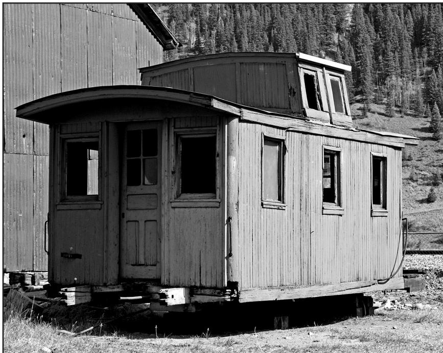
Silverton Northern's 2 axle caboose #1005 had been stored in the Durango yard until this summer. Seen here in back of the SN engine house in Silverton on October 2, 2010, it should soon move inside for restoration. This car was originally built in 1880 as D&RG #17, and is similar to caboose #59 at the CRRM in Golden.
